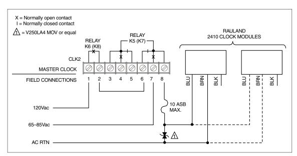
Figure B-10 Wiring Rauland 2410 Digital Clocks for 120Vac
